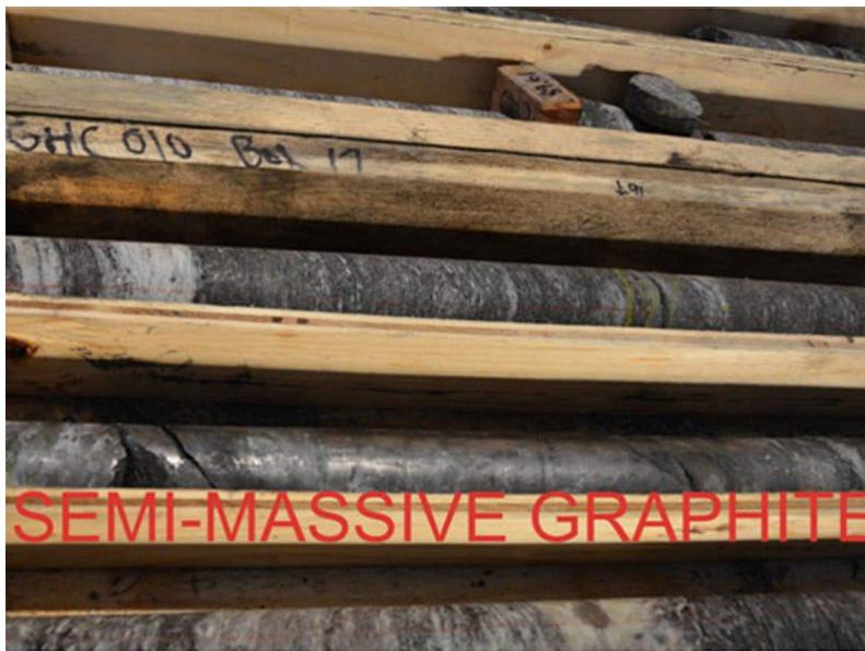
Mineralisation at the Graphite Creek project is characterised by massive and semi-massive graphite segregations. Image courtesy of Graphite One Resources.
